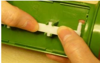
6) Pass the "uprights" of the treadle "goal-post" through the holes in the base-plate and snap them over the pins in the treadle "T-arm".
