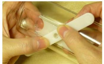
15) Snap the transparent cover into place, making sure all six buttons are engaged.
