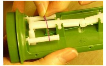
9) Now you can test the sensitivity of the trip-weight and adjust it by sliding the spring along the pegs. A 3g trip-weight is achieved when the spring is approximately aligned with the anchor pillar. (Note how this also doubles as a stop for the "T-arm".)
