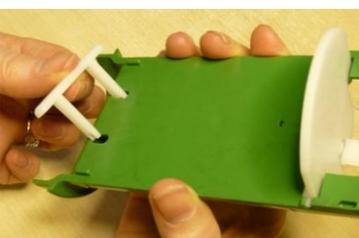
6) Unsnap the treadle "T-arm" out of its clips.
