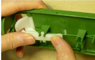
5) Put the pin of the treadle "T-arm" into the socket of the "short-arm" and then snap it into its clips.
