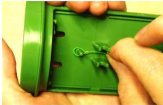
4) Snap the treadle "short-arm" into its clips. It doesn't matter whether the socket is on the left or right-hand side.
