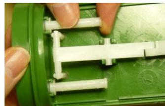
8) Slide the purple trip-weight spring onto the two pegs.
