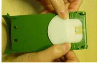
2) Hook the large loop of the green door spring through the notch in the "shark fin" on the door.
