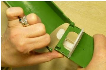
2) Remove the transparent base by sliding a finger-nail down one edge and then pulling the tab beneath the door lock.
