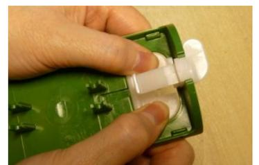
10) Push the door lock and catch together down the slot in the base-plate.
