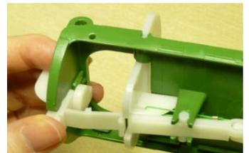
12) Check the trip-weight again and ensure that the door closes smoothly and fully when tripped. (You may need to bend the catch slightly to reduce the friction on the "shark fin" as the door closes.
